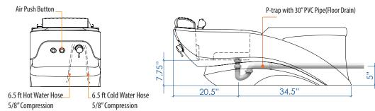
**Wall Drain:** Flex drain pipe extended 2ft from the back of the basin **Floor Drain:** Drain pipe & bushing extended 3" from the back of the basin
